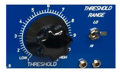
.THRESHOLD: this is the control for the level where the compressors acts Threshold is steped ( rotary switch).
